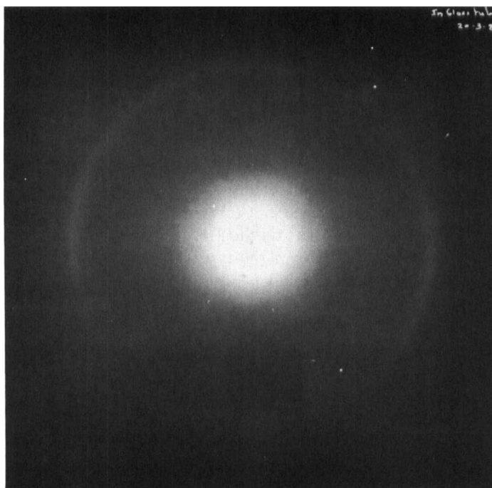
Figure 8. X-ray diffraction pattern of the lyotropic liquid-crystalline mesophases of dye 1 in water (32.5 wt% dye).
